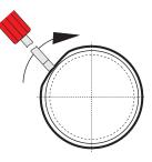
**3.2.** With your finger, hold the section of the seal already pressed in from step 3.1. (This helps prevent loops.) Use the seat assembly tool to press a short section of the seal in the direction of your finger. Continue around the circumference to install the seal into the groove.
