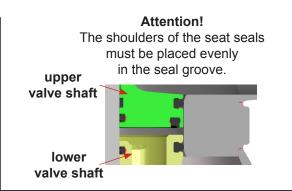
**3.1.** Press a short section of the seal into the groove.
