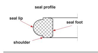
1. Provide the seal shoulder with a thin layer of grease.
