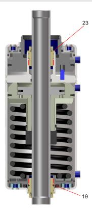
fig. 23: Actuator screw
